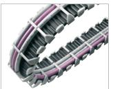
Where more of space is needed, the take-up capacity can be doubled by laying the cables on both sides. In this case every second side-part is simply attached the other way round.
