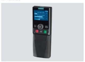
A handheld version of the IOP can be ordered for mobile use. In addition to the IOP, this includes a housing with rechargeable batteries, charging unit and RS232 connecting cable. The charging unit is supplied with connector adapters for Europe, the US and UK. When the batteries are fully charged, the operating time is up to 8 hours.
