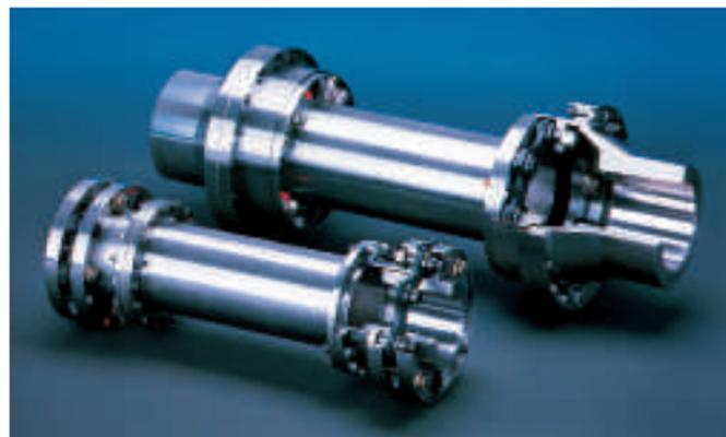
The steel disk couplings of the construction series Raflex® belong to the torsionally stiff, flexible shaft connections. Like the well-established curved tooth couplings, these power transmission elements are completely made from metal. Contrary to the curved tooth couplings, they do not need lubrication and are hence maintenance-free.
